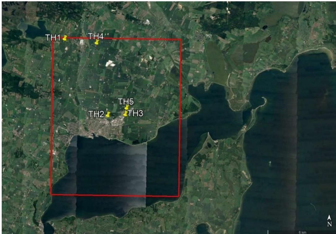
Figure 6.1. Map of the Thisted-area with the model domain indicated by the red rectangle and boreholes indicated by yellow pin marks. TH2 is the production well and TH3 and TH5 are injection wells. TH1 and TH4 are older hydrocarbon exploration wells.
