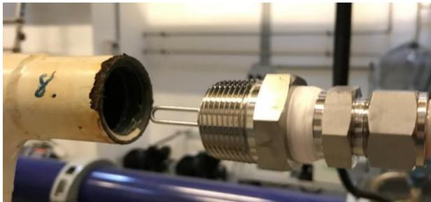
Figure 6. Wire-loop for corrosion rate measurement by ER technique.
