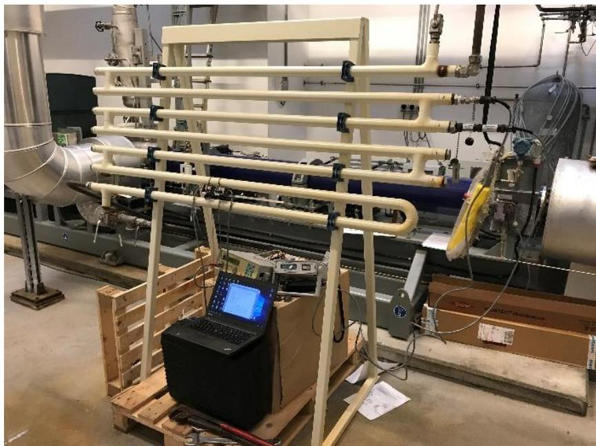
Figure 3. Side-stream loop for corrosion monitoring in pressurized line downstream the injection pump.
