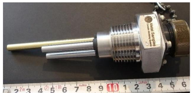
Figure 5. Galvanic probe with brass and carbon steel coupons.
