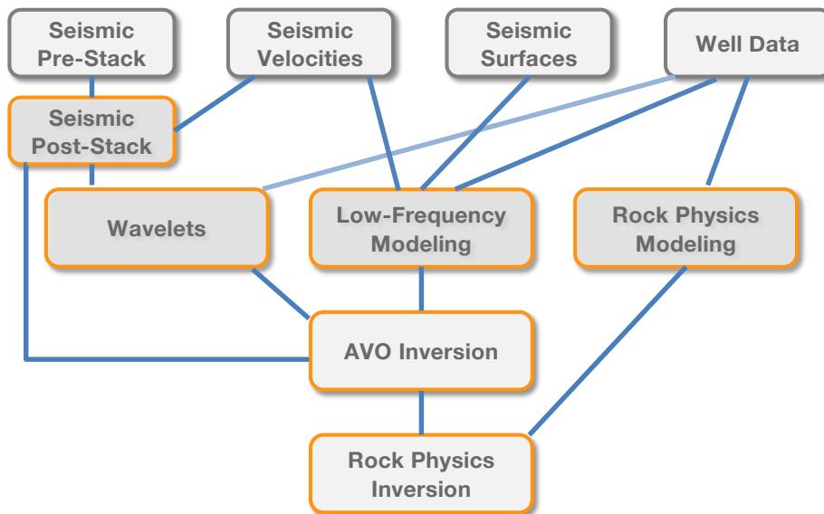
**Figure 4.1:** Flow chart for the general workflow. First row lists the input data. The steps towards the rock physics inversion through the AVO inversion are marked with orange outlines.
